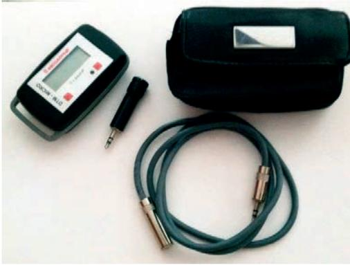
The **MEGADYNE DTM-MICRO** is used to determine the tension of a drive belt, by measuring the frequency of the static belt. Employing the latest microprocessor technology, offers ease of use with precise measurement results. Measuring the acoustic frequency, this device can be used for all types of Power Transmission belts:
