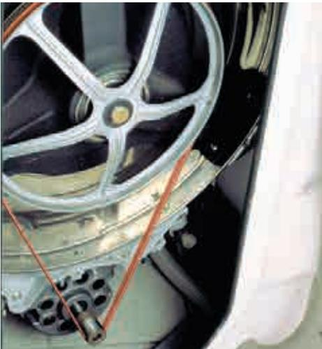
On request, special elastic Megarib belts can be manufactured in polyurethane with a semi-elastic tension member. They can be fitted on fix centre drives, reducing noise and vibrations. The absence of a tensioning mechanism, offers additional cost savings.
