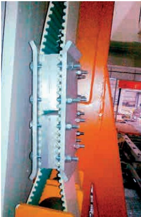
**MEGALINEAR** can be supplied as open length rolls, (standard roll lengths are 50 or 100 metres) or as endless jointed belts, available in a wide range of solutions with numerous tooth design: Imperial profile, metric profile with or without guide, parabolic profile, flat...
