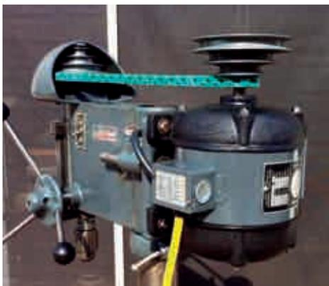
**ACCU\_LINK** adjustable V-Belts are the ideal replacement substitute for conventional rubber V-Belts.
